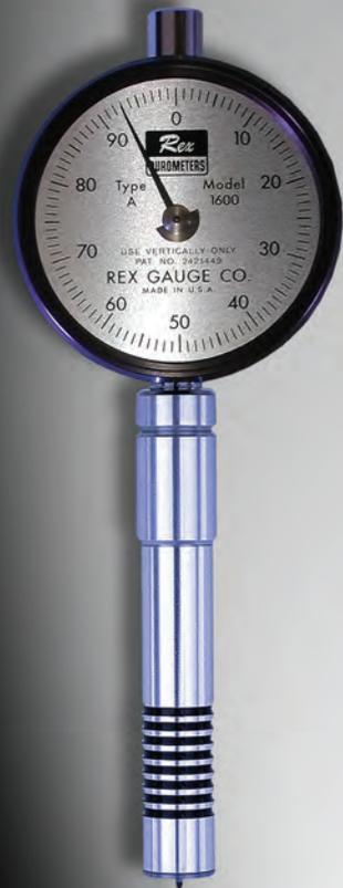
Conforms to ASTM D-2240
